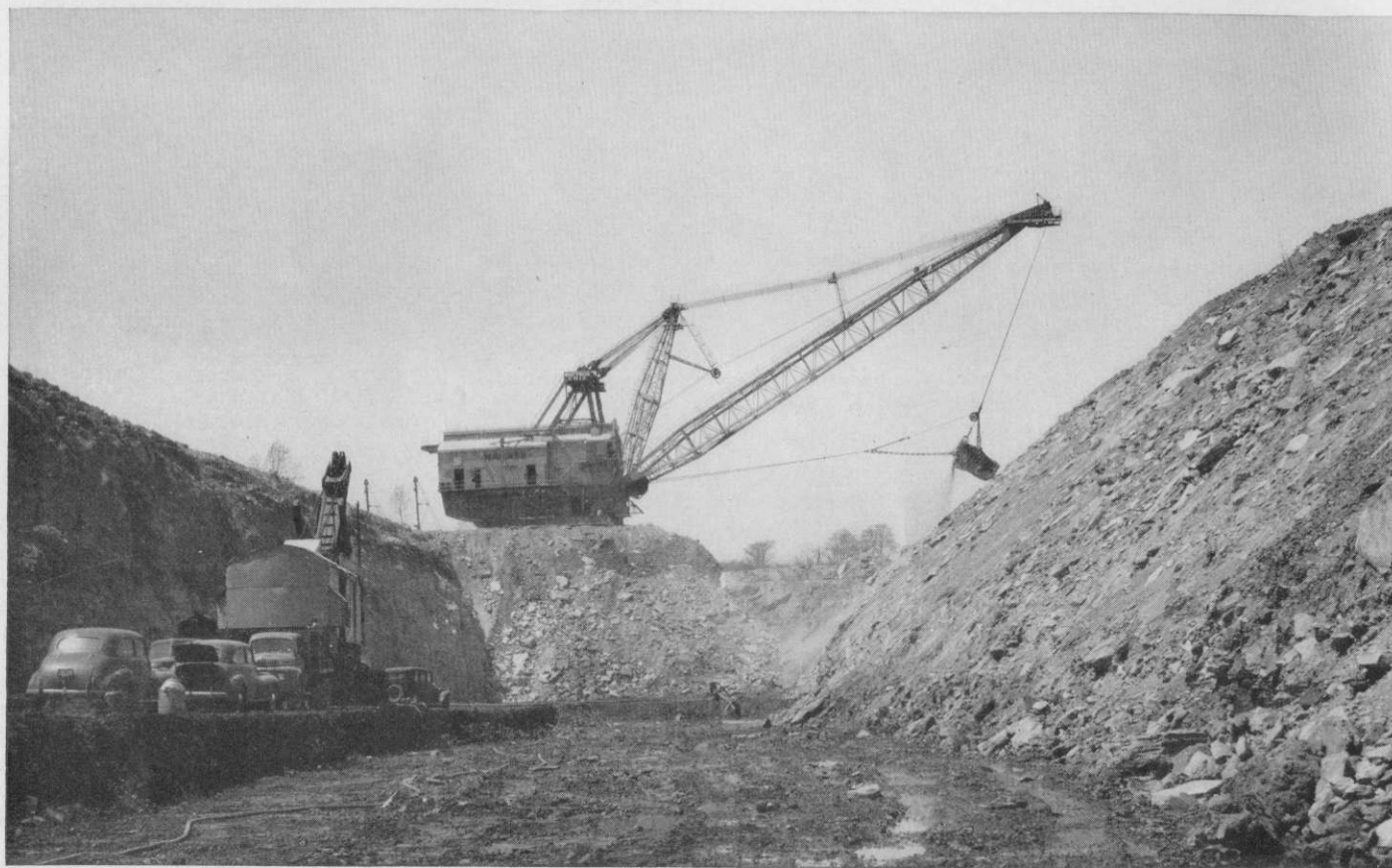
The dragline—modern method of mining strip beds—here removes the overburden from a coal vein. This piece of machinery costs from $300,000 to $1,000,000 and serves the purpose of digging a trench 40 to 50 feet wide with a depth of 10 to 90 feet. A ponderous instrument, the dragline awkwardly but efficiently swings its shovel back and forth carrying load after load of shale, stone and dirt away from the immediate mining area.
