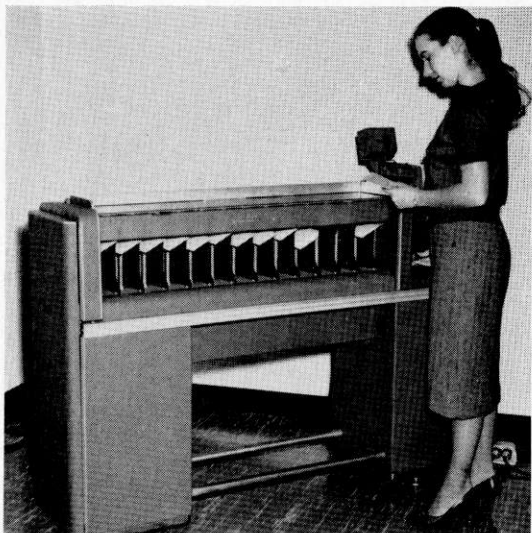
The IBM Electronic Sorter automatically arranges cards in alphabetical or numerical sequence, sorts out cards for statistical use; for example, the number of boats with in-board motors of a given horsepower in a certain area, if such information were needed.
