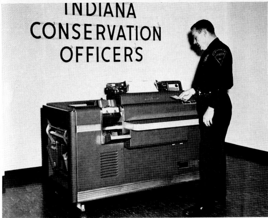
Officer Joseph Planck, Enforcement Division central office, checks a test registration from the IBM Printer. The Printer decodes the perforations in the Key punch file card, translates them into legible symbols, and prints the certificates of registration at the rate of 25 per minute.
